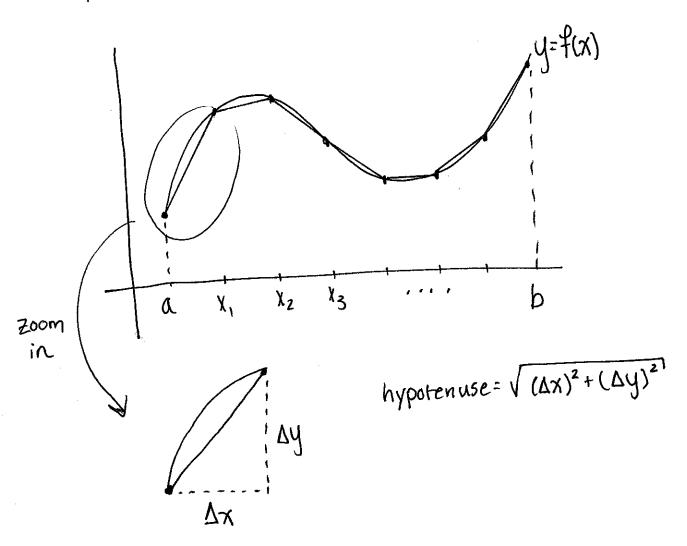
The not completely rigorous way to get Arc Length.  $\Delta x \approx dx$   $\Delta y \approx dy$
