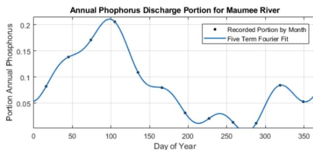
$$f(t) = a_0 + a_1 \cos(t*w) + b_1 \sin(t*w) + a_2 \cos(2*t*w) + b_2 \sin(2*t*w) + a_3 \cos(3*t*w) + b_3 \sin(3*t*w) + a_4 \cos(4*t*w) + b_4 \sin(4*t*w) + a_5 \cos(5*t*w) + b_5 \sin(5*t*w)$$
