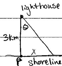
Since the light makes 4 rev/min,  $\frac{d\theta}{dt} = \frac{4 \text{ rev}}{\text{min}} \cdot \frac{2\pi \text{ rad}}{\text{rev}} \cdot \frac{60 \text{ min}}{\text{hr}} = \frac{8\pi \cdot 60 \text{ rad}}{\text{hr}}$
